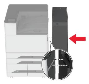
11 Open the trifold/Z-fold finisher door, use the screw to secure the finisher to the printer, and then close the finisher door.
