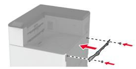
**16** Insert the paper transport, and then use the screws to secure it.
