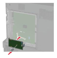
**8** Connect the ISP extended cable to the ISP connector on the controller board.
