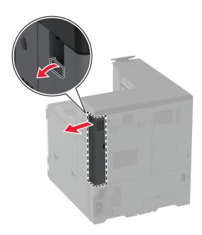
**3** Using a flat-head screwdriver, remove the controller board access cover.
