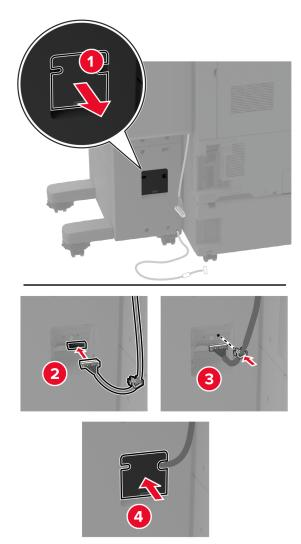
Connect the finisher cable to the rear of the printer.
