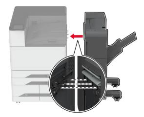
**13** Adjust the leveling screws to make sure that all sides of the finisher have the same height as the printer.
