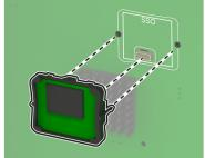
**6** Attach the controller board access cover.
