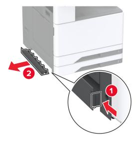
**6** Pull out the lifting handle on the left side of the printer.
