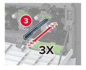
Put the printhead wiper back into place.
