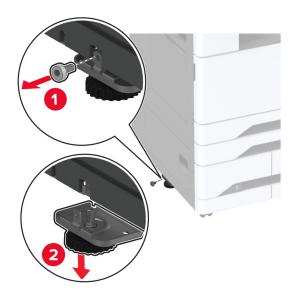
**5** Attach the docking bracket to the printer.
