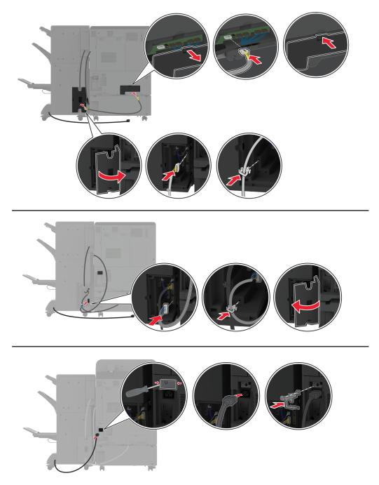
**27** Connect the power cord to the printer, and then to the electrical outlet.
