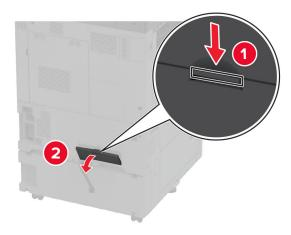
Connect the tray connector to the printer, and then attach the cover.
