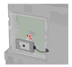
Attach the hard disk connector cable to the controller board.
