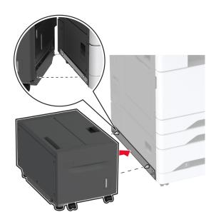
Connect the tray connector to the printer.
