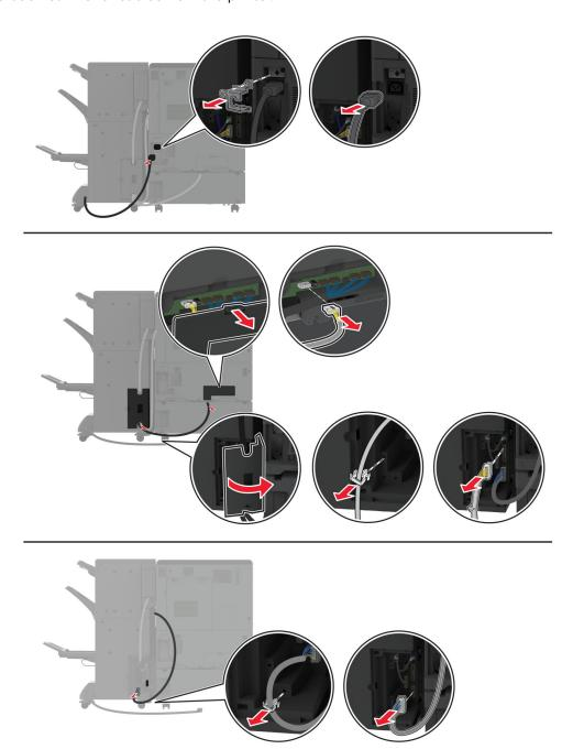
**4** Open the booklet finisher door, use a flat-head screwdriver to remove the screw and metal bracket, and then close the door.
