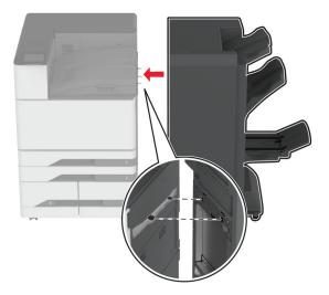
**24** Open the finisher door, use the screw to secure the finisher to the printer, and then close the door.
