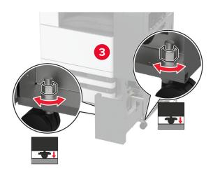
**13** Adjust the leveling screws to make sure that the rear of the finisher has the same height as the printer.
