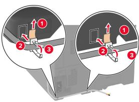
11 Connect the finisher cable to the printer.
