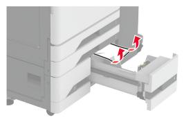
In tandem trays, pull out handle C, and then open the inner cover.
