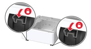
**5** Remove the option installation cover under the left side of the printer.
