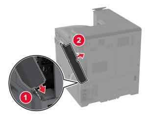
Attach the brackets at the bottom of the finisher.
