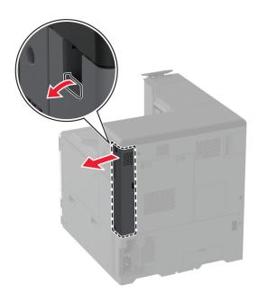
Using a flat-head screwdriver, remove the used controller board access cover.
