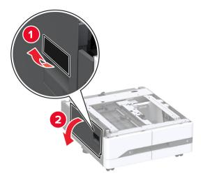
**7** Remove the option installation cover under the left side of the printer.
