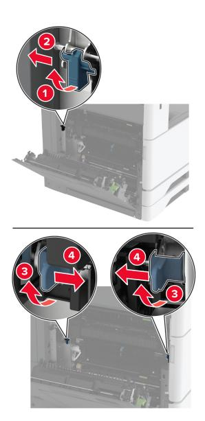
Remove the used fuser.
