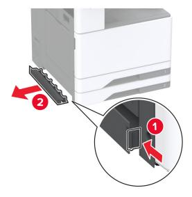
**8** Pull out the lifting handle on the left side of the printer.
