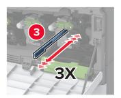
8 Put the printhead wiper back into place.
