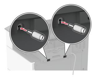
**10** Secure the finisher cable to the printer.
