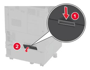
Secure the locking bracket to the printer, and then attach the cover.
