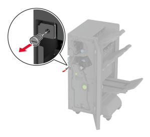
Attach the finisher to the printer.
