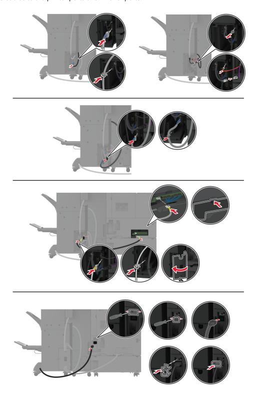
19 Connect the printer and finisher power cords to the printer and the finisher, and then to the electrical outlet.
