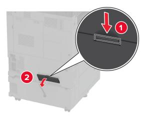
**13** Connect the tray connector to the printer, and then attach the cover.
