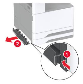
**7** Pull out the lifting handle on the left side of the printer.
