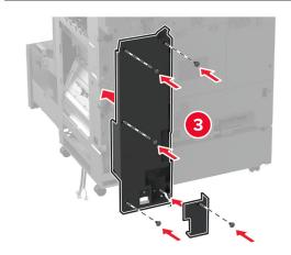
Attach the wrench to the trifold/Z-fold finisher.
