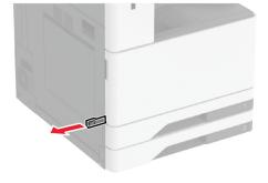
**8** Align the printer with the optional tray, and then lower the printer into place.
