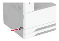
**7** Align the printer with the spacer, and then lower the printer into place.
