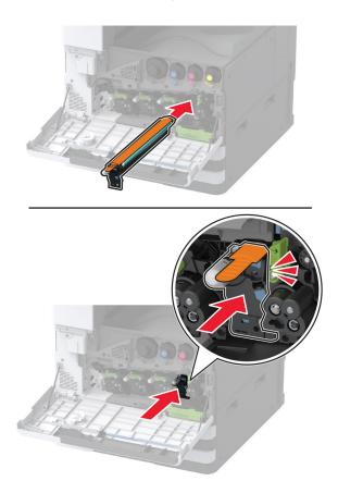
**7** Remove the packing material, and then lock the new photoconductor unit.
