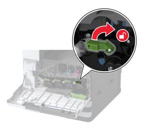
Remove the used photoconductor unit.
