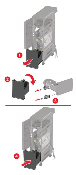
**9** Using a flat-head screwdriver, attach the installation bracket for the trifold/Z-fold finisher, remove the screw, and then close the finisher door.
