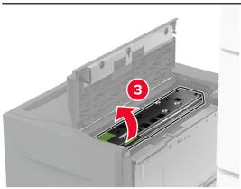
Locate and remove the used roller kit.
